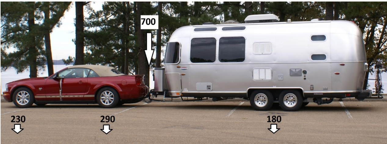
This is how 700 pounds of hitch weight is distributed on this combination.
