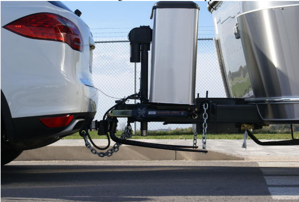
This is how 700 pounds of hitch weight is distributed on this combination.
